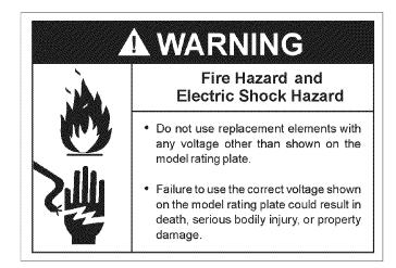
Replacement elements must (1) be the same voltage and (2) no greater wattage than listed on the model rating plate affixed to the water heater.
